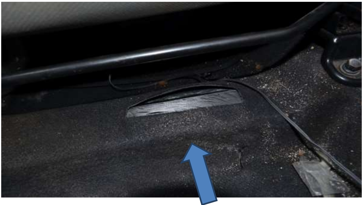
The VIN number located on the base plate of the front passenger's seat. This number has been ground away.
